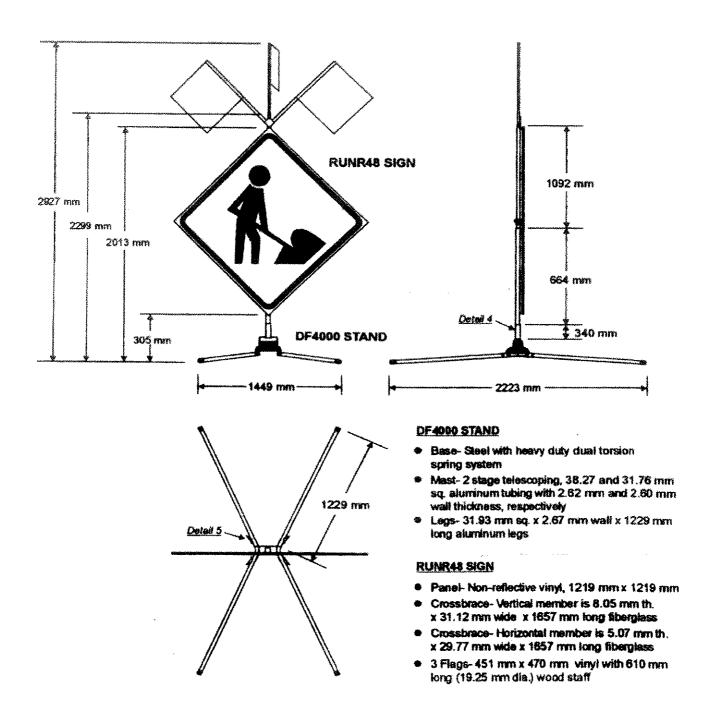
Figure 4. System Nos. 58 and 59 Sign Support Details, Test D-30
