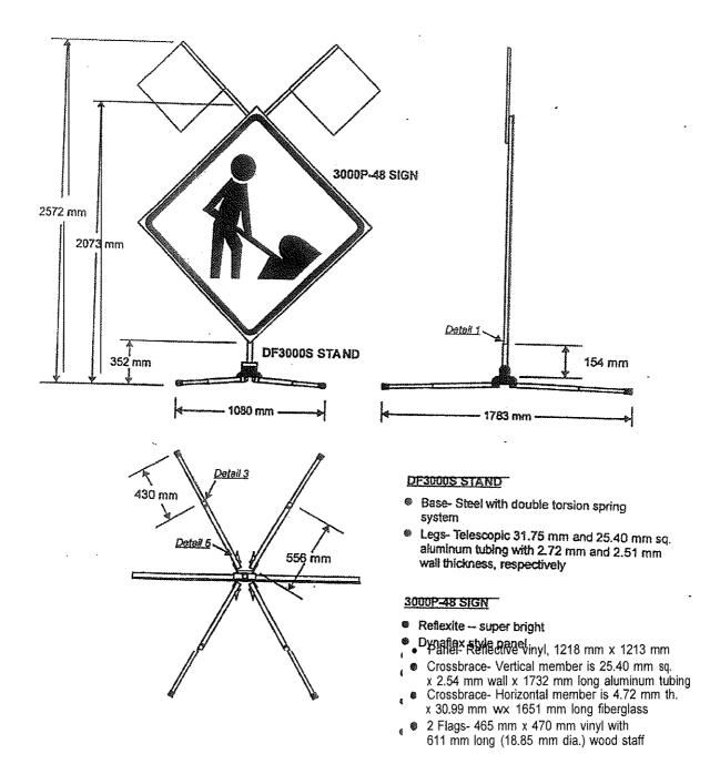
Figure 19. System No. 13 Sign Support Details, Test D-7
