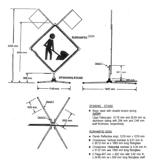
Figure 41. System No. 24 Sign Support Details, Test D-12
