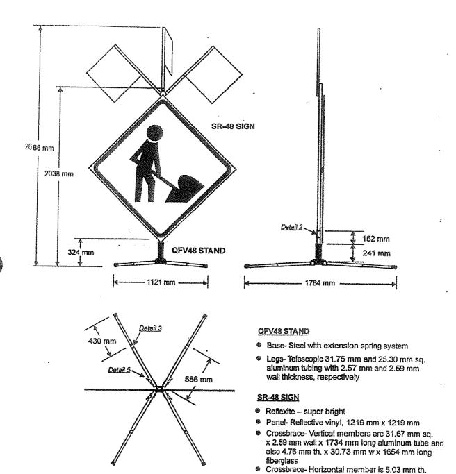
Figure 27. System No. 17 Sign Support Details, Test D-9
