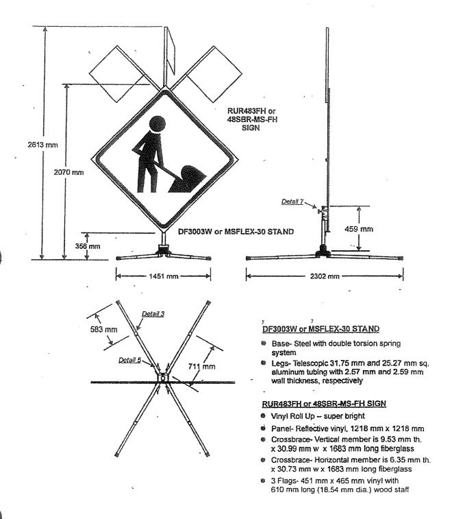
Figure 23. System No. 15 Sign Support Details, Test D-8
