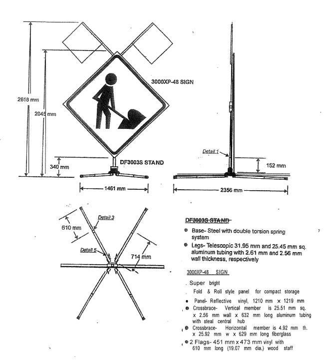
Figure 3 1. System No. 19 Sign Support Details, Test D- 10
