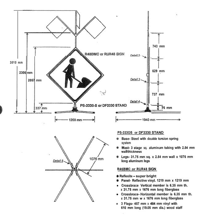
Figure 17. System No. 12 Sign Support Details, Test D-6
