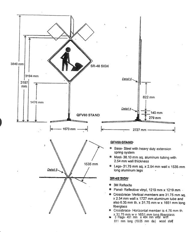
Figure 12. System Nos. 9 and 10 Sign Support Details, Test D-5
