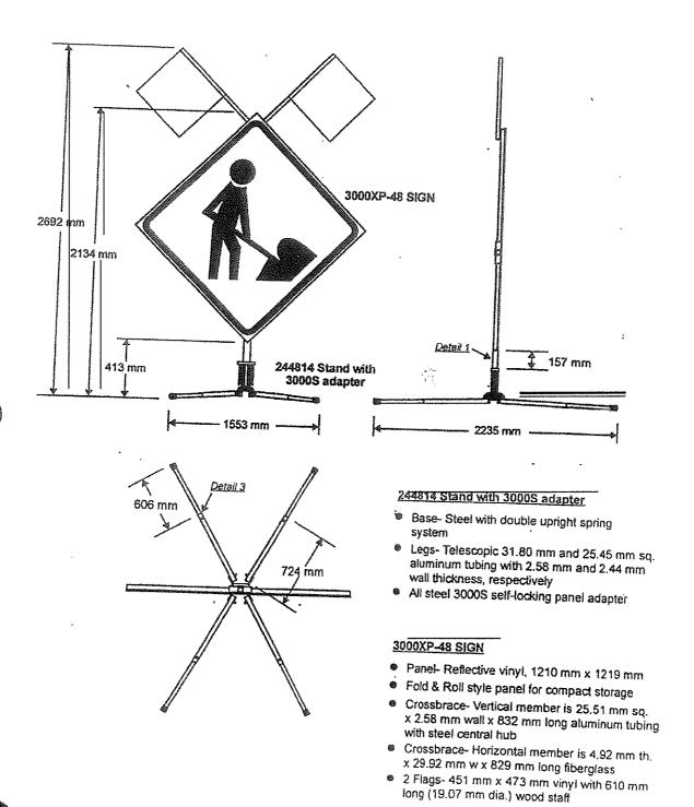
Figure 33. System No. 20 Sign Support Details, Test D- 10
