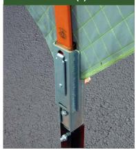
Signs are held in place by capturing the bottom rectangular plastic pocket on standard roll-up signs. A spring-loaded catch locks the sign into the base, a lift of the lever releases the sign. The channel style panel holder locks the roll-up sign to the stand with a lever actuated pin. The rollup sign's vertical fiberglass rib, with predrilled locking hole, slides down into channel opening and engages a locking pin. Used with our 400 series signs.
