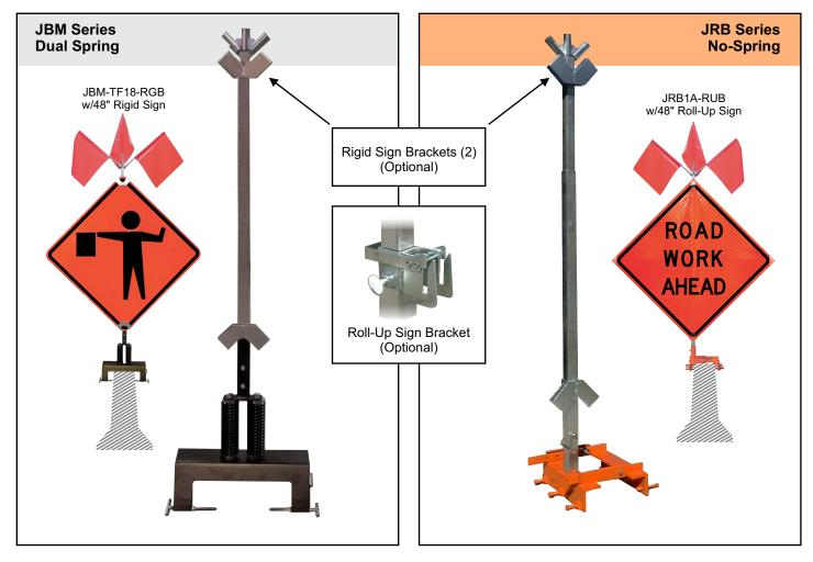
Barrier mount sign stands are designed to display 36" and 48" rigid and roll-up signs on concrete highway barriers. Units are firmly affixed using multiple heavy duty screws. All models feature aluminum masts with either rigid or roll-up brackets depending on model and sign type. The **JBM-TF18** series features a double spring system for added stability in windy conditions.
