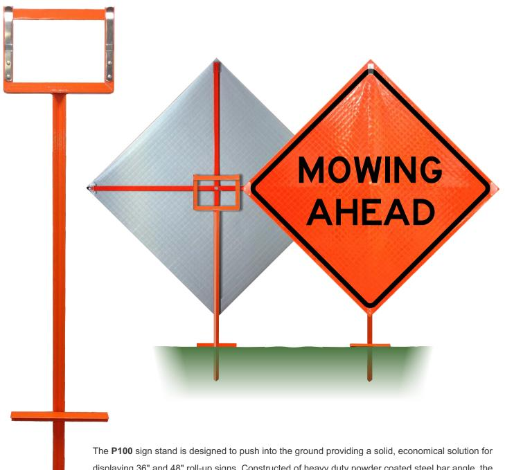
displaying 36" and 48" roll-up signs. Constructed of heavy duty powder coated steel bar angle, the **P100** features steel spring clips that holds the sign securely and has a cross piece at the bottom for pushing the stand into the ground by foot . 12" x 2" x 57", weight: 6 lbs.
